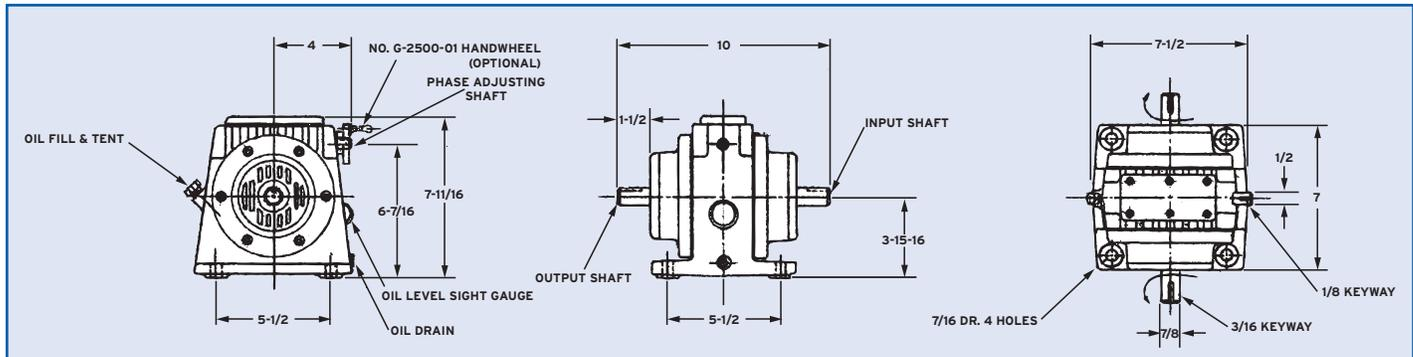
One Rotation of Adjustment Shaft, while running or stopped, provides approximately  $3\frac{3}{4}^\circ$  Radial Movement of Output Shaft (96:1 Ratio)
