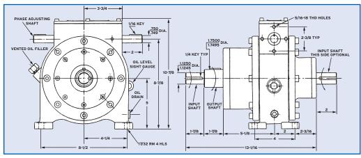
One Rotation of Adjustment Shaft, while running or stopped, provides approximately 5½° Radial Movement of Output Shaft (66:66:1 Ratio)
